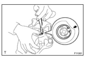
(c) Using snap ring pliers, install the snap ring. HINT:
