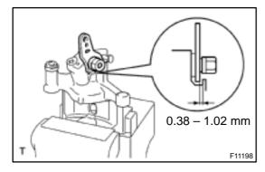
(c) Check that there is clearance between the parking brake crank and caliper.
