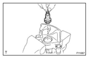
(b) Install the adjusting bolt assembly into the cylinder.
